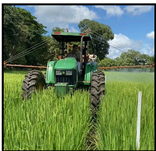
Figure 1. Tractor and Spray Boom (SB) used during spraying.
