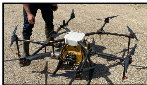
Figure 2. Unmanned aerial vehicle (UAV) used during spraying.
