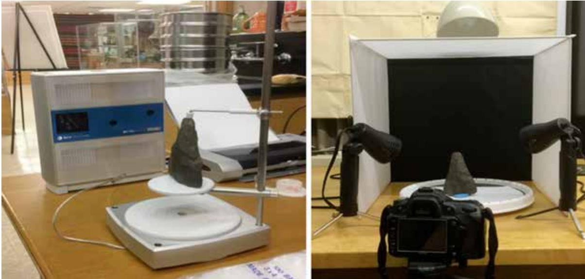
**Figure 11:** Left, NextEngine 3-D scanner; right, photogrammetric workstation.
