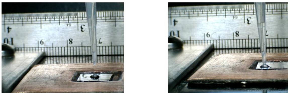
Figure S2. Electrochemical cell setup used for measuring \text{Mn}_{12}\text{-(methacrylate)-Si(100)} .
