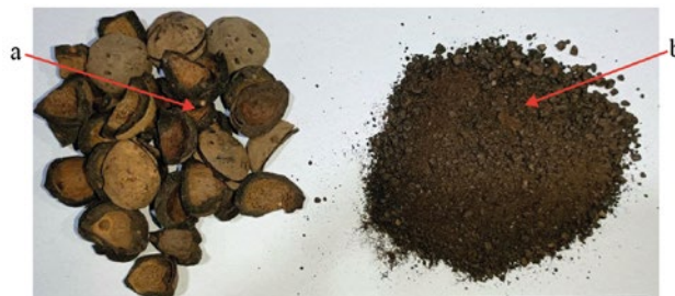
Fig.13. Comparison of the nutshell of the macaw fruit palm ( Acrocomia sp.) a) not ground and b) ground.
