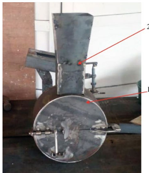
Fig.2. Mill shell and hopper built.
