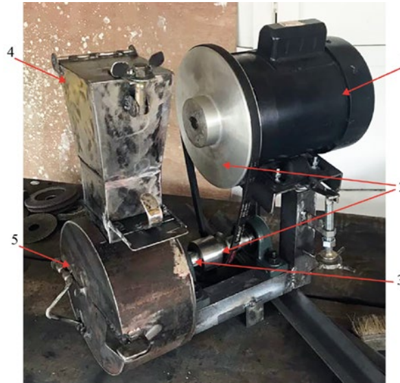
Fig.5. Real Assembly of the mill shell and mill base.
