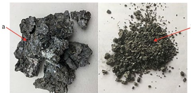
Fig. 14. Comparison of aluminum slag a) not ground and b) ground.
