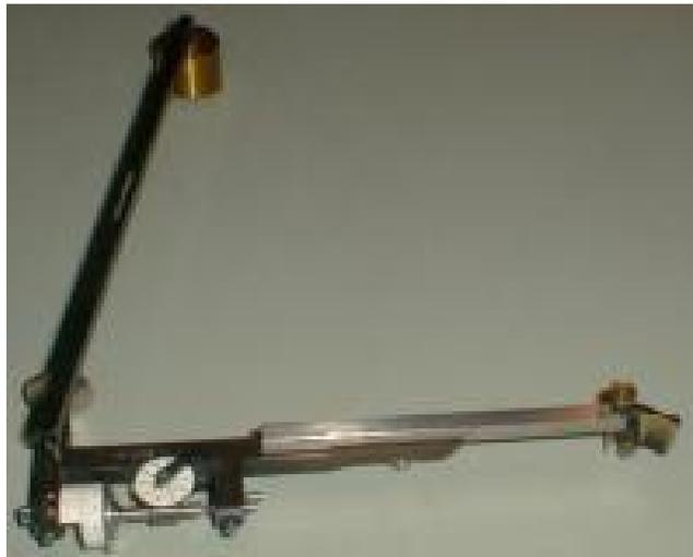
The planimeter is fixed at the origin  $O$  (but free to pivot) and has a hinge at  $P$ , as indicated in the figure below. The end of the tracer arm  $PQ$  moves counterclockwise around the region  $R$ . A small wheel at  $Q$  is perpendicular to  $PQ$  and a scale is marked on it to measure how much it rolls while  $Q$  traces out the boundary of the region  $R$ .
