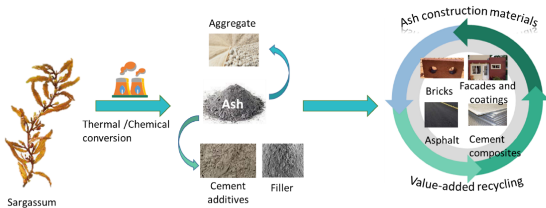
Figure 3. Upcycling of sargassum ash into construction materials. Source: self made
