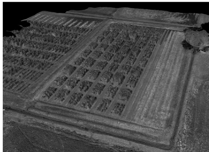
Figure 3. Three-dimensional mesh of the experimental plots generated from UAS imagery using Pix4D. Cañas, Guanacaste. 2023.
