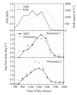
Fig. 3. Diurnal courses of atmospheric saturation deficit (ASD), photosynthetically active radiation (PAR), and sap flow rate measured using the HDT and potometry in two *Hyeronima alchorneoides* trees during the first day of observations.
