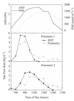
Fig. 2. Diurnal courses of atmospheric saturation deficit (ASD), photosynthetically active radiation (PAR) and sap flow rate measured using the HDT and potometry in two *Ochroma lagopus* trees during the first day of observations.
