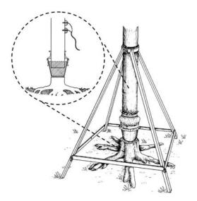
Fig. 1. Schematic diagram of a potometer system consisting of an excised tree with its base immersed in a water reservoir. The tree stem was suspended with a large metallic frame. The inset shows a closer view of the potometer tree on which Granier probes were implanted at approximately 1 m above the cut.
