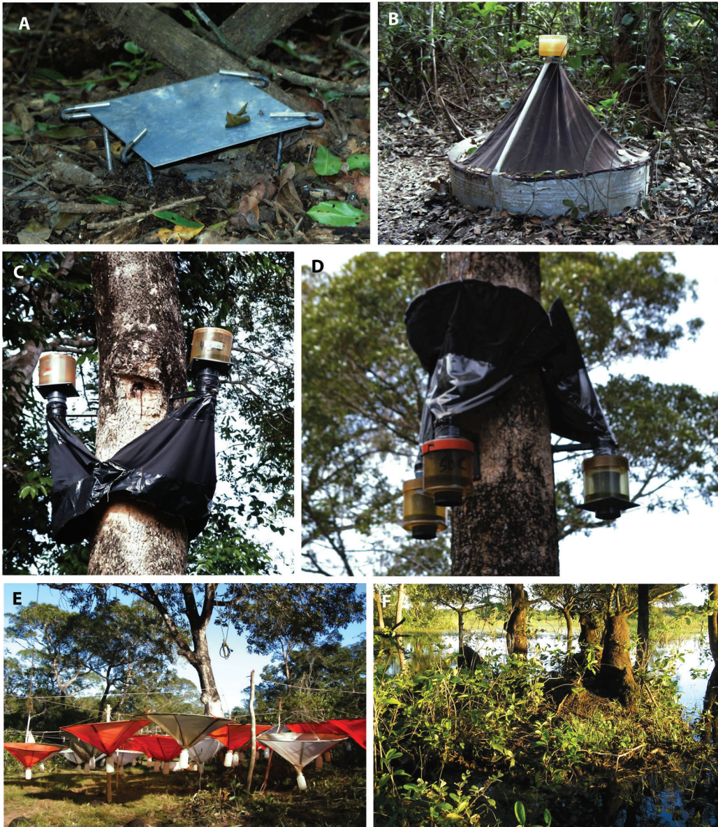
Fig. 1. Methods employed in the sampling of Pseudoscorpiones in a seasonally flooded V. divergens Pohl. ( Vochysiaceae ) monodominant forest in the Brazilian Pantanal: A: Pitfall traps; B: Soil photoelector; C: Trunk photoelector (soil to canopy); D: Trunk photoelector (canopy to soil); E: Fogging (canopy fogging); F: Murundus associated with termite mounds within the forest (Pictures: Leandro Battirola).
