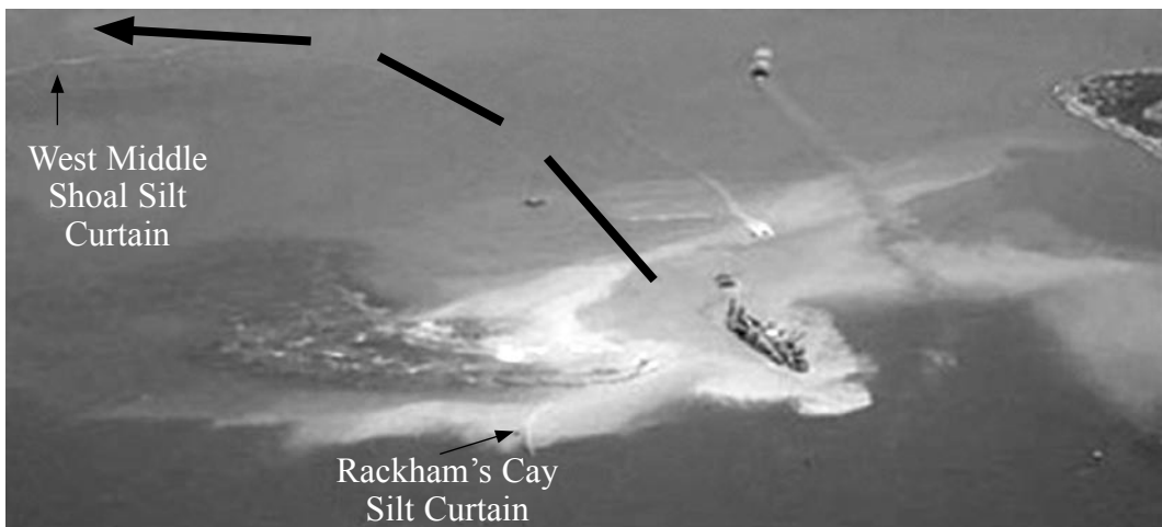
Fig. 4. Positions of silt curtains and movement of sediment plume, 14 June 2002. Red arrow: direction of plume movement three days earlier.
