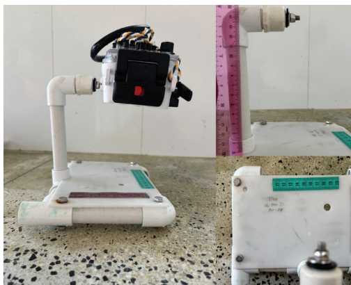
Fig. 2. Portable photographic station used for standardized imaging of coral fragments underwater. A. Lateral view of the PVC frame and mounted digital camera. B. Lateral view showing the fixed distance between the camera mount and acrylic platform. C. Top view of the acrylic platform with the reference scale used for planar area measurements.
